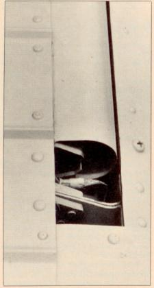
A new gap seal closes off airflow between the elevator and stabilizer providing just a touch more low-speed pitch control.
